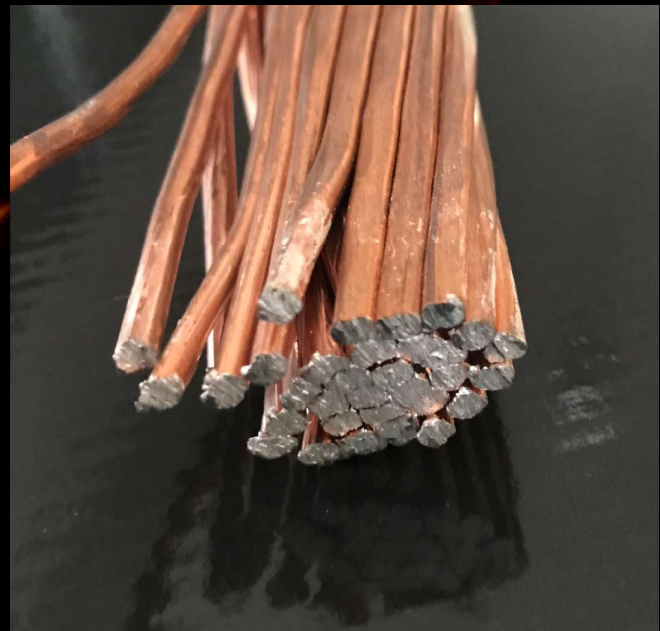
An example of copper clad aluminium conductors.
