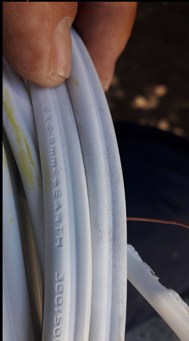
Flat twin and earth cable without a SANS specification or SABS mark
