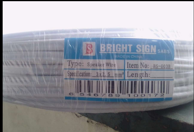
Flat twin and earth cable labelled as speaker wire.
